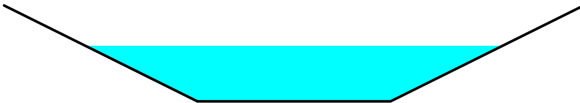
Reach 2R: Diversion Swale
